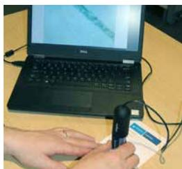
10. Analyze the sample with the 100x magnification field microscope.
