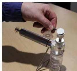
4. Separate the funnel from the patch supporter and install a filter patch with ink grid up. (If the patch has an ink grid).
