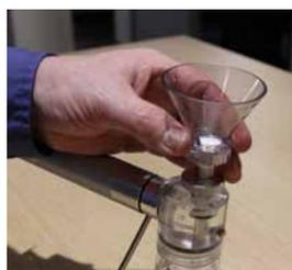
5. Reattach the funnel to the filter patch base with filter patch. Twist lock the funnel to the base.
