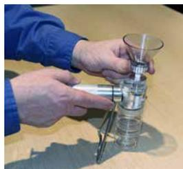
1. Assemble waste bottle, funnel-patch assembly, and vacuum pump to form the sample processing assembly. Tighten the vacuum pump o-ring on the funnel-patch assembly tube by turning the aluminum locking device.
