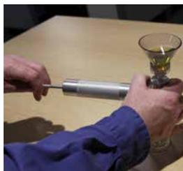
7. Draw the sample fluid through the patch by pulling on the vacuum pump handle.
