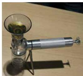
6. Agitate the sample fluid bottle and pour 25ml into the funnel. 25ml is denoted by the first line on the funnel (closest to the patch).
