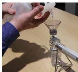
3. Rinse the funnel-patch assembly with the filtered solvent to remove background contamination. The patch should not be in place for this process.
