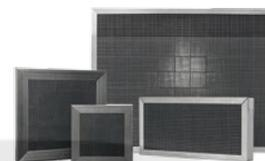
The Viledon® HM® modules are an assembly of Versacomb™ media housed in either a plastic or metallic frame for removing gas phase contaminants from outdoor or recirculated air. The module is available in nominal depths of one, two, four and six inches as standard. Viledon® HM® modules are designed to fit in a side-access filter rack or a Type 8 filter frame, and are available with or without a header.
