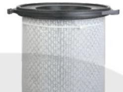
The CPSs are made from a fully synthetic PES filter medium, that excels particularly in terms of very high air-permeability measuring approx. 3880 l/m<sup>2</sup>·s and a mean pore size of approx. 50 µm. Fine particles can penetrate the filter medium, while coarse ones are arrested.
