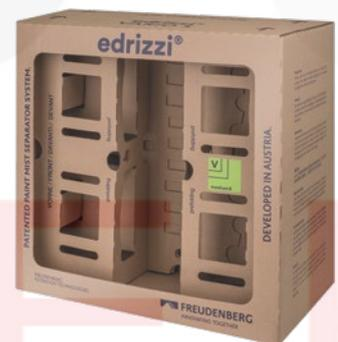
Made from fire retardant corrugated board, the patented edrizzi® paint mist separators have a capacity of up to 25 kg with a separation efficiency of up to 97%. The system saves both time and costs. The paint mist separators can be quickly replaced and disposed of at low cost in incineration plants. They complete our portfolio of multi-stage filter systems.
