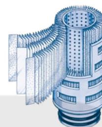
In the production of filter cartridges, Viledon® novatexx spunbonded nonwovens serve as "spacers" between the pleats on the face side and as a drainage layer on the clean side. The performance profiles of the media concerned can be very specifically designed to requirements. The nonwovens involved can be easily pleated together with the membrane without damaging the latter.
