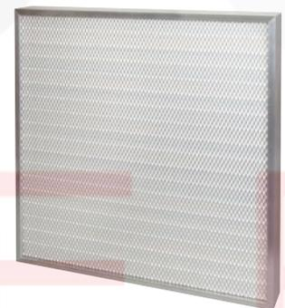
For air filtration at temperatures above 100 °C up to a maximum of 385 °C, the Viledon® high-temperature filters are the right choice. The silicone-free filter elements meet particularly stringent requirements for air purity, process dependability and cost-efficiency. The pleated filter media are made from special, thermally stable micro-glass-fiber papers.
